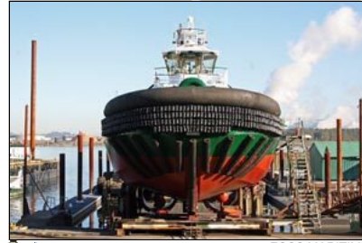
PHOTO: FOSSE This diesel-electric hybrid tugboat, believed to be the first of its kind in the world and is being made for the ports of Los Angeles and Long Beach, is being built by Seattle-based Foss Maritime at its shipyard in Rainier, Ore.
